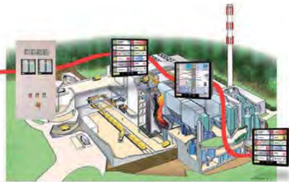
RS485 Bus / 1 km / fitted with 64 modules as a maximum
