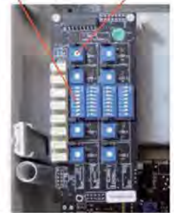
8 inputs card (4 possible cards per stage)
