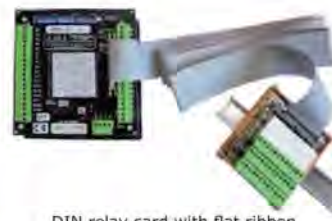
DIN relay card with flat ribbon
